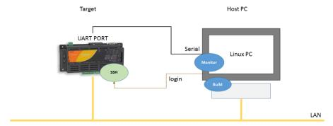
Example 2) with one development host PC to build software (or source code edit), use a serial monitor for target with other Windows PCs.
