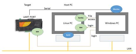
Example 3) to use as a development host PC by installing virtual OS system (VM Ware, Virtual BOX etc.) into Windows OS, and installing Linux OS from the virtual system.
