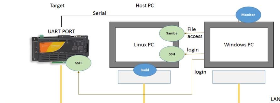
**Example 3) to use as a development host PC by installing virtual OS system (VM Ware, Virtual BOX etc.) into Windows OS, and installing Linux OS from the virtual system.**
