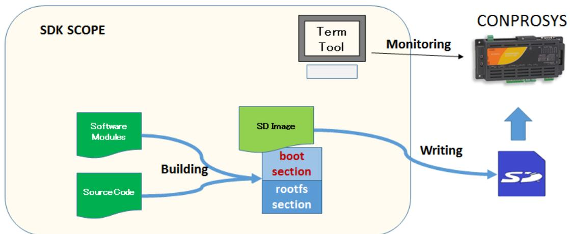
This SDK generates software modules in the cross-build development on the Host PC.
