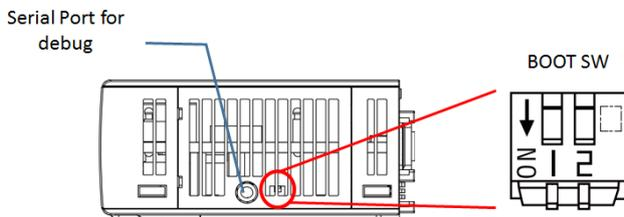
Insert the SD card you made in "**Create a SD card for start-up (page 33)**" and turn on the product power. Without the SD card, booting starts from built-in NOR FLASH.
