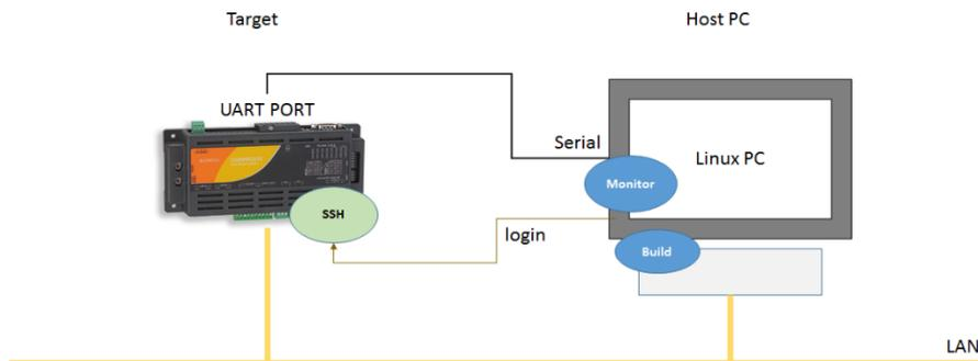
**Example 2) with one development host PC to build software (or source code edit), use a serial monitor for target with other Windows PCs.**
