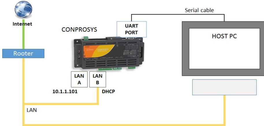
In the default setting, 10.1.1.101 is set in LAN A port (I/F on Linux is eth0), and DHCP network is set in LAN B port (I/F on Linux is eth1). Also, you can connect LAN cable to CONPROSYS directly from the host PC to access 10.1.1.101- IP address via network.
