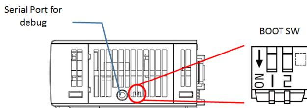
By connecting a serial cable from the host PC to CONPROSYS through the serial port (3.5Φ MINI-JACK), you can login from the console to the product. See the setting details below.
