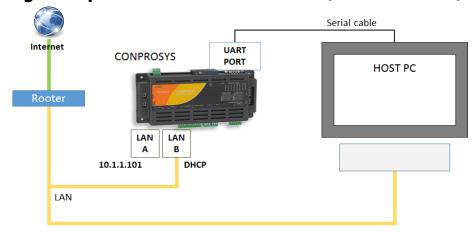
In the default setting, 10.1.1.101 is set in LAN A port (I/F on Linux is eth0), and DHCP network is set in LAN B port (I/F on Linux is eth1). Also, you can connect LAN cable to CONPROSYS directly from the host PC to access 10.1.1.101- IP address via network.
