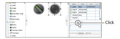
The list of usable devices are displayed. Simply selecting the device from the list can link data. Choose "CPU DO02" from the Device Tree and click the [OK].
