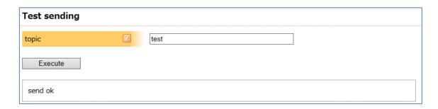
When the Test sending has been completed, go to [Service] from the Setting on the CONPROSYS WEB Setting. Select the [Enable] in the "MQTT Client" and click the "Set". Save the settings to ROM of the controller and reboot the product.
