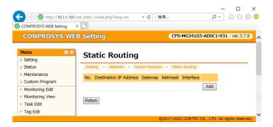
\*Click Add on the screen to proceed to the screen for adding settings to "Static Routing".
