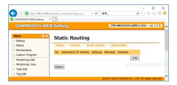
Click the [Add] button to add a setting to "Static Routing". Up to 32 settings are possible.
