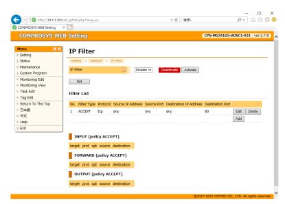
\*\*Click Add on the screen to proceed to the screen for adding settings to "IP Filter".
