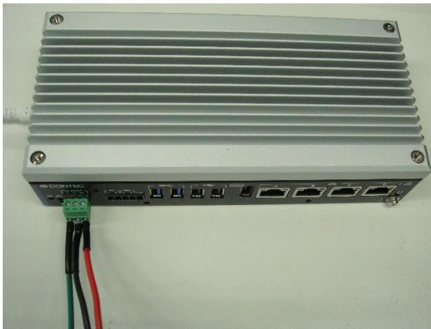
1. Set the setting switch (SW1) on the side of the chassis to ON so that the system will boot in recovery mode when the power is turned on.
