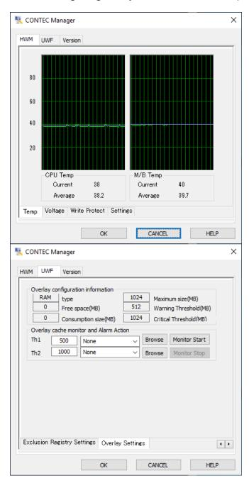
Monitor hardware status such as the CPU temperature, the M/B temperature and so on. If it exceeds the set threshold, the set alarm action will be activated.
