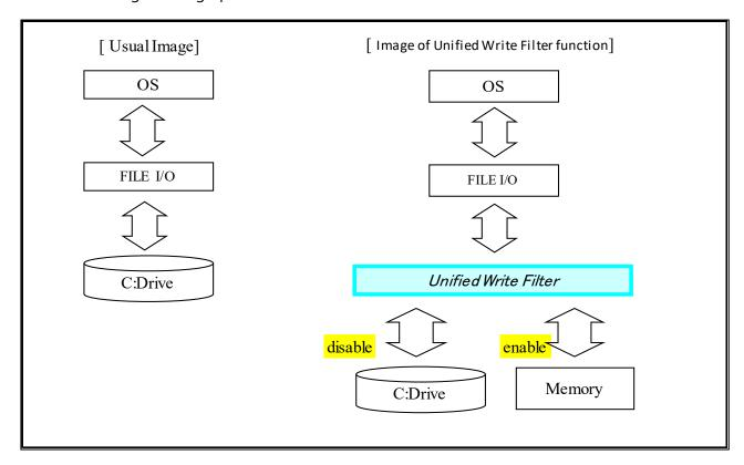
The following explains the method for setting write protection for the C drive using UWF manager (uwfmgr.exe).
