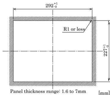
Figure 4.2. FPD-M21VT-AC [10.4inch] Panel Cut Dimensions
