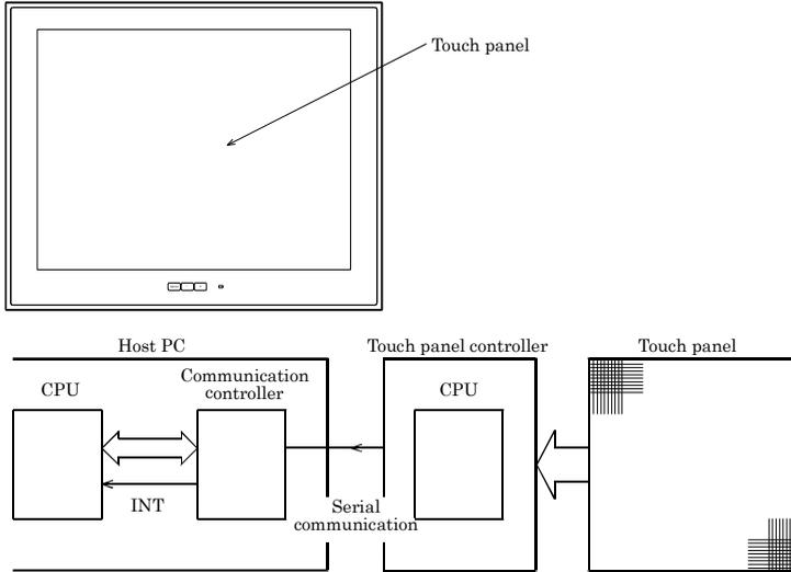
**Figure 9.1. Touch Panel and Block Diagram**
