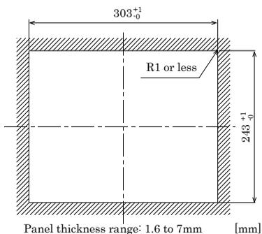
Figure 4.3. FPD-L21ST-AC [12.1inch] Panel Cut Dimensions and Stud Hole Positions
