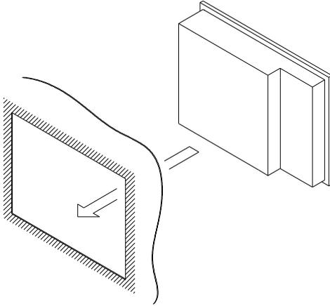
Figure 4.5. Attaching the Fitting Used to Attach to the Main Unit < 1 / 2 >
