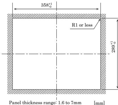
Figure 4.4. FPD-H21XT-AC [15inch] Panel Cut Dimensions and Stud Hole Positions
