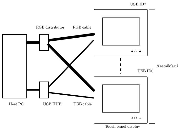
**Figure 9.2. Example of connection of a USB multi-touch panel**
