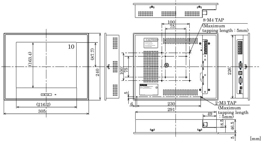
Figure 3.1. Outside Dimensions of Main Unit (FPD-M21VT-AC)
