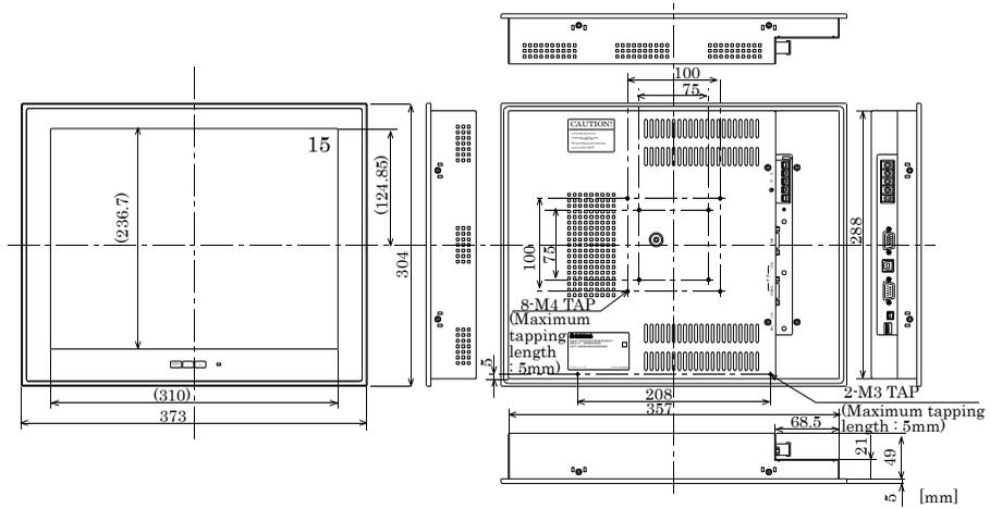
Figure 3.3. Outside Dimensions of Main Unit (FPD-H21XT-AC)
