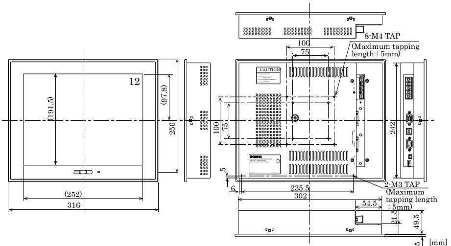
Figure 3.2. Outside Dimensions of Main Unit (FPD-L21ST-AC)
