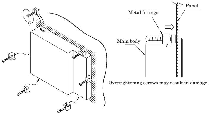
Figure 4.5. Attaching the Fitting Used to Attach to the Main Unit < 2 / 2 >
