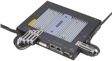
Figure 3.5. Using example of cable clamp
