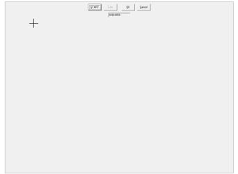
② Press [START] button and touch the center of the cross shown on the screen. Note that data would be inputted when you release the touch.
