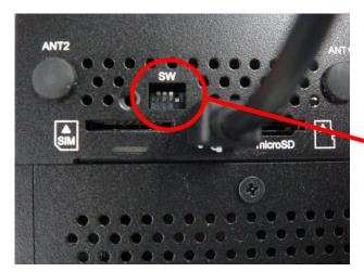
Set the DIPSW 4PIN on the side of the chassis to ON so that the system will watchdog-off when the power is turned on.
