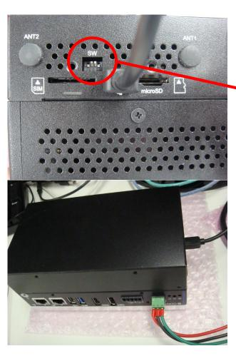
Set the DIPSW 1PIN on the side of the chassis to ON so that the system will boot in recovery mode when the power is turned on. Also set the DIPSW 4PIN to ON so that the system will boot with watchdog-off.
