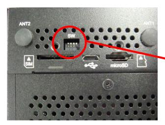
11. After turning off the power, set back the DIPSW 4PIN on the side of the chassis to OFF and switch to normal booting (eMMC).
