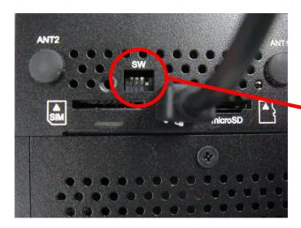
After turning off the power, set back the DIP SW 1PIN on the side of the chassis to OFF and switch to normal booting (eMMC).
