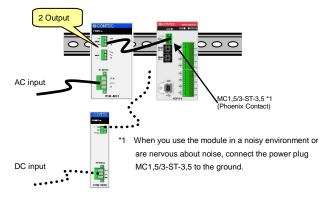
For the power supply for installation on a DIN rail, use the connector MC 1,5/3-ST-3,5 (Phoenix Contact).
