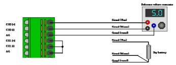
Moreover, you should connect the module by using a 2-core shielded cable in situations where the signal source is at a considerable distance from the module or the noise immunity must be increased.
