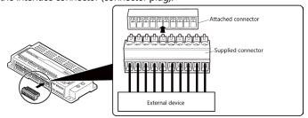
[Attached connector]: European type terminal 3.5 pitch 10-pin jack connector
