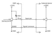
\*Input pins are indicated as DI xx. xx corresponds to input bits.
