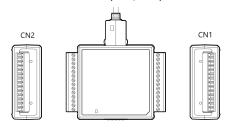
Layout on the Interface Connector(CN1, CN2)
