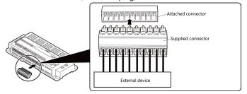
[Attached connector]: European type terminal 3.5 pitch 10-pin jack
