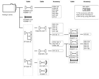
\*1 Two sets of cables are necessary to use the DT-G2E-32.
