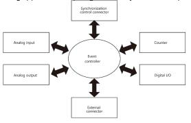
Scenario 1: Analog input and output synchronized with an external dock signal. Scenario 2: Analog input performed whenever the counter value reaches the set value.
