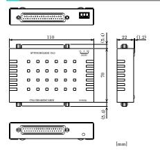
This product is purposed to add buffer amplifier function to CONTEC analog input boards.
