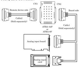
\*1: To obtain an effective buffer amp connection, connect this unit near to the analog input board. Using a 0.5 m Shield Cable is recommended.
