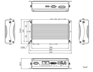
When you fasten the bundled attachment fittings to be fixed to the body, you should use the attached screws  $(M4\,x\,10).\,Otherwise, the length\,(L)\,from\,the\,surface\,of\,the\,cabinet\,to\,the\,screw\,tip\,should\,be\,5mm\,or\,less.$
