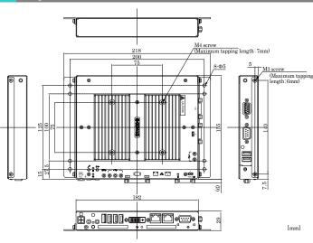
\*1 The length (L) from the tip of M4 boss to the M4 screw tip should be 5mm or less. If not doing so, it may be exactly fixed.
