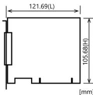
The standard outside dimension (L) is the distance from the end of the board to the outer surface of the slot cover.
