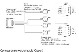
Connection Conversion Cable for Serial I/O (37P→9P×4, 250mm)
