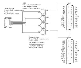
Connection conversion cable (Option) Connection Conversion Cable for RS-232C (37P→25P×4, 250mm)
