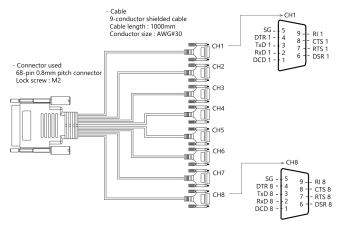
Connector used 9-pin D-SUB, male connector Thumb screw : UNC#4-40(inch screw) Applicable connectors 17JE-13090-02(D8C) (mfd. by DDK, Female)
