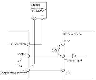
Example connection of Output and TTL level input (Current sink type) < CPSN-DO-08BL >
