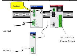
When using the power supply installable on DIN rail, please use the connector MC1,5/3-ST-3,5(Phoenix Contact).
