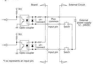
The signal inputs are isolated by opto-couplers (ready to accept current sinking output signals). The product therefore requires an external power supply to drive the inputs. The power requirement for each input pin is about 5.1 mA at 24 VDC (about 2.6 mA at 12 VDC).
