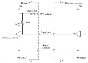
\* I-xx represents an input pin. One polyswitch is connected for Vcc(+5V) terminal.
