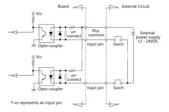
The signal inputs are isolated by opto-couplers (ready to accept current sinking output signals). The product therefore requires an external power supply to drive the inputs. The power requirement for each input pin is about 5.1 mA at 24 VDC (about 2.6 mA at 12 VDC).
