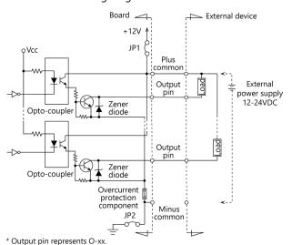
The signal output section is an opto-coupler isolated, open-collector output (current sink type).
