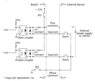
The input circuits of interface blocks of this product are illustrated in Figure. Connect the input signals to a device which can be current-driven, such as a switch or transistor output device.
