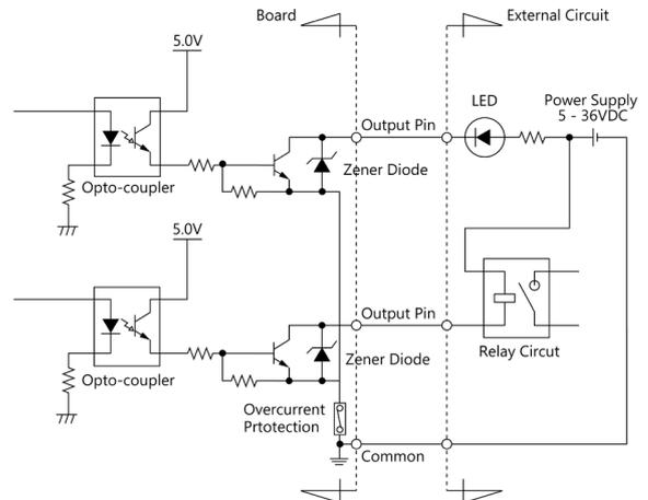
The signal output section is an opto-coupler isolated, open-collector output (current sink type). The rated output current per channel is 100mA at maximum. The output section can also be connected to a TTL level input as it uses a low-saturated transistor for output.
