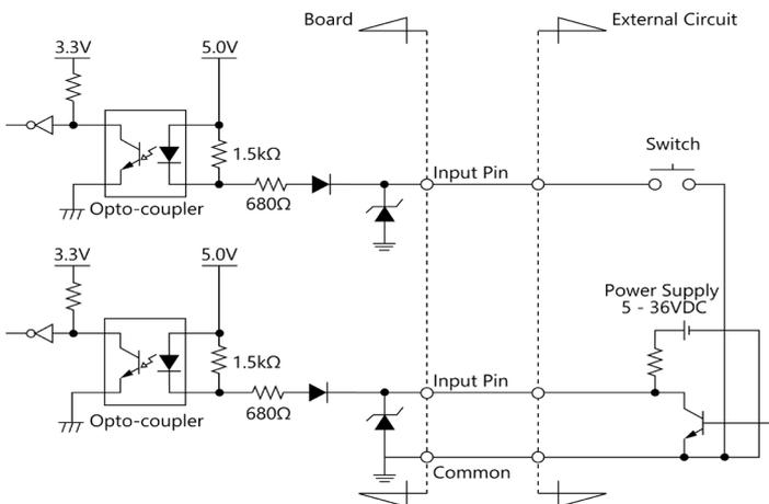
The signal inputs are isolated by opto-couplers (ready to accept current sinking output signals). The current requirement to turn on the input is 6.4mA and a leakage current of less than 0.57mA is required to turn off the input. A zener diode is connected to each input for protection from surge voltages.
