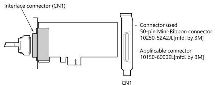
Layout on the Interface Connector(CN1)
