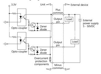
The signal output section is an opto-coupler isolated open-collector output (current sink type), driving the output section requires an external power supply.
