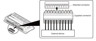
[Attached connector]: European type terminal 3.5 pitch 10-pin jack connector [Supplied connector]: European type terminal 3.5 pitch 10-pin plug connector [Compatible cable]: AWG28 - 16
