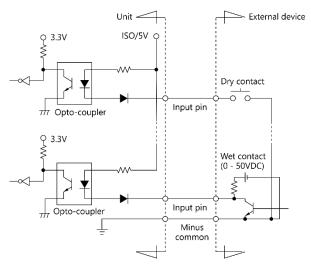
Each input channel accepts either dry contact or 0-50 VDC wet contact inputs. The signal input section is a Optocoupler isolated input (current sink output compatible). To turn the input ON, a current of 1.15 mA or more must flow, and to turn the input OFF, the leakage current must be 0.16 mA or less. In addition, as the power to run the opto-couplers for input section is supplied internally (5VDC), no external power supply is required.
