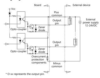
The signal output section is an opto-coupler isolated, open-collector output (current sink type). Driving the output section requires an external power supply.
