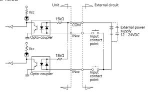
The signal input section consists of an Opto-coupler isolated input (compatible with both current sink output and current source output). An external power supply is therefore required to drive the input section of
