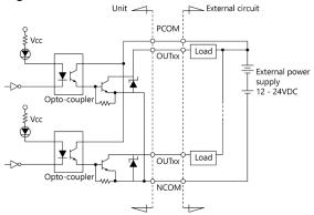
The signal output section consists of an Optocoupler isolated open collector output (current sink type). An external power supply is therefore required to drive the output section of this product.
