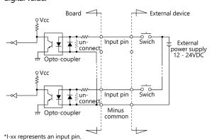
The signal inputs are isolated by opto-couplers (corresponding to the current source output). The product therefore requires an external power supply to drive the inputs. The power requirement for each input pin is about 5.1 mA at 24 VDC (about 2.6 mA at 12 VDC).
