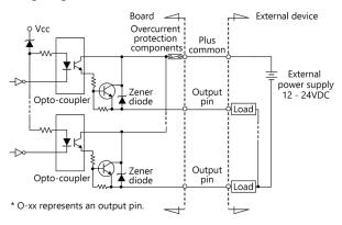
The signal output section is an opto-coupler isolated output (current source type). Driving the output section requires an external power supply.
