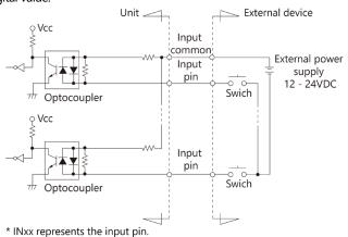
The input specification is fixation from 12 - 24VDC for this product. The signal inputs are isolated by opto-couplers (Both of current sink and source outputs supported). The board therefore requires an external power supply to drive the inputs. The power capacity required for driving each input channel is about 4 mA when the signal voltage is 12VDC.
