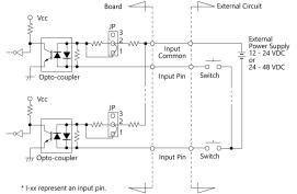
For each input channel, use the corresponding jumper to select a voltage range of 12 - 24 or 24 - 48 VDC depending on the voltage of the input
