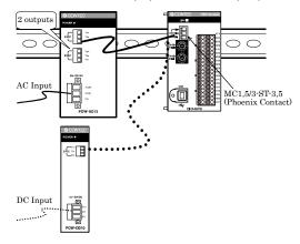
When using the power supply installable on DIN rail, please use the connector MC1,5/3-ST-3,5 (Phoenix Contact).
