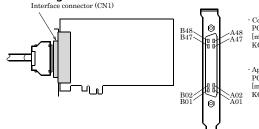
Connector used PCR-E96LMD+ equivalent to it [mfd. by HONDA TSUSHIN KOGYO CO., LTD.]
