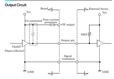
\* O-xx represents an output pin. One polyswitch is connected for Vcc(+5V) terminal.
