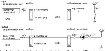
Resistor value should be adjusted according to the specification of the LED to use and the desired intensity level.
