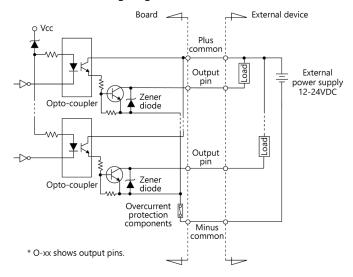
The signal output section is an opto-coupler isolated, open-collector output (current sink type). Driving the output section requires an external power supply. The rated output current per channel is 100mA at maximum. The output section can also be connected to a TTL level input as it uses a low-saturated transistor for output. The residual voltage (low-level voltage) between the collector and emitter with the output on is 0.5V or less at an output current within 50mA or at most
