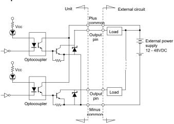
Figure above shows the output circuit for the interface section of this product. The signal output section consists of an Optocoupler isolated open collector output (current sink type). An external power supply is therefore required to drive the output section of this unit.
