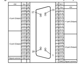
O-00 - O-37 32 output signal pins. Connect these pins to the input signal pins of the external
