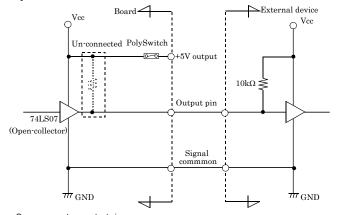
\* O-xx represents an output pin. One polyswitch is connected for Vcc(+5V) terminal.
