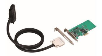
This product is an expansion adapter that connects the optional expansion chassis, ECH-PCI-BE Series to a PC to extend a PCI Express bus expansion slot in the PC, thereby providing additional PCI bus expansion slots.
