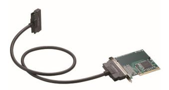
The EAD(PCI)BE or EAD(LPCI)BE is an expansion adapter that connects the optional expansion chassis ECH-PCI-BE to a PC to extend a PCI bus expansion slot in the PC, thereby providing additional PCI bus expansion slots.
