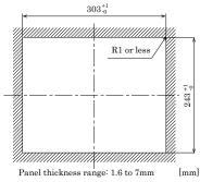
FPD-H21XT-AC [15inch] Panel Cut Dimensions and Stud Hole Positions
