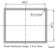
FPD-L21ST-AC [12.1inch] Panel Cut Dimensions and Stud Hole Positions
