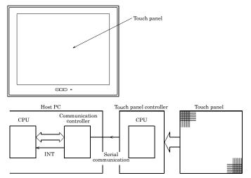
Data input at the touch panel is processed by the touch panel controller and passed to the host PC via the serial port on the CPU in the controller.
