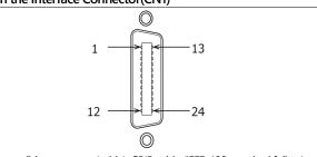
Compatible connector (cable): GPIB cable (IEEE-488 standard follow)
