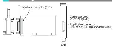
Layout on the Interface Connector(CN1)
