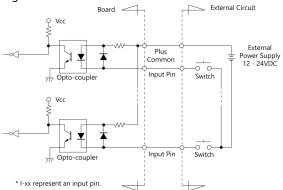
The input circuits of interface blocks of the PI-128L(PCI)H are illustrated in the figure above.
